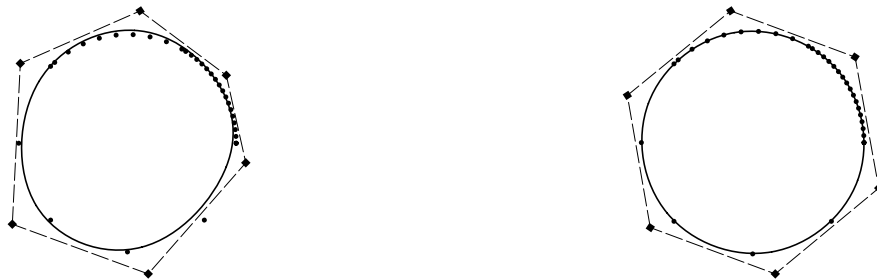
(c) The fitting curve generated by SDM in 3 iterations. (d) The fitting curve generated by SDM in 10 iterations.
