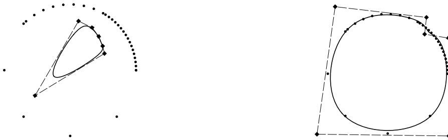
(a) Data points on a circle with an initial B-spline spline (b) The fitting curve generated by PDM in 50 iterations. curve.
