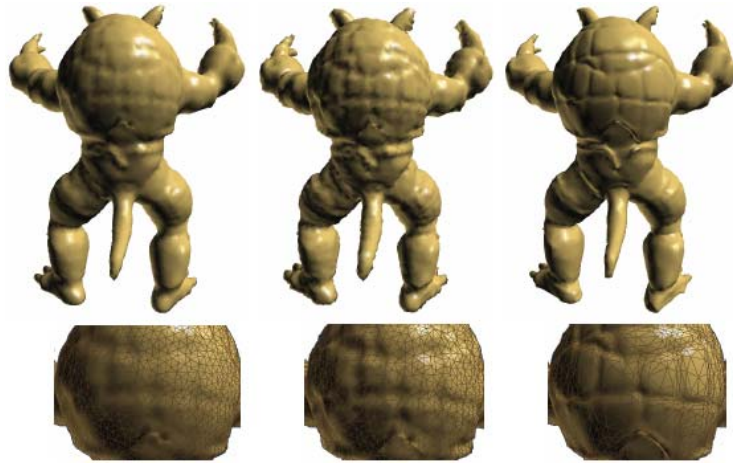
Fig. 8: Comparison with Guskov et al.'s approach [7]. Left: a resampling mesh of Armadillo model; Middle: result generated by Guskov's approach; Right: result by vertex flowing.
